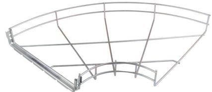
**Technical:****Product Type** Pre-Fabricated Bend**Width** 300mm**Height** 60mm**Weight** 0.64 Kgs**Angle** 90°**Material** Pre-Galvanised Steel (Zinc Coated)**Colour/Finish** Self Colour**Supplied With** Pre-Installed FastConnect Coupler
