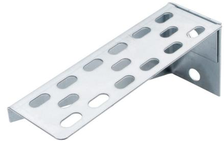
**Technical:****Product Type** Cantilever Arm**Width** 50mm**Height** 70mm**Length** 150mm**Weight** 0.30 Kgs**Gauge** Light Duty**Material** Pre-Galvanised Steel (Zinc Coated)**Colour/Finish** Self Colour**Standards** BS EN 10346:2015
