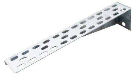
**Technical:****Product Type** Cantilever Arm**Width** 50mm**Height** 70mm**Length** 300mm**Weight** 0.70 Kgs**Gauge** Light Duty**Material** Pre-Galvanised Steel (Zinc Coated)**Colour/Finish** Self Colour**Standards** BS EN 10346:2015
