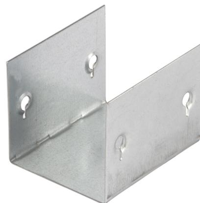
**Technical:****Product Type** Coupler**Width** 50mm**Height** 50mm**Weight** 0.15 Kgs**Material** Pre-Galvanised Steel (Zinc Coated)**Colour/Finish** Self Colour**Standards** BS EN 50085-2-1 2006; BS EN 10346:2015**Trunking Weights:**
