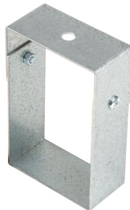
**Technical:****Product Type** Hanger**Width** 100mm**Depth** 45mm**Height** 100mm**Dimensions** Suspension Size (mm): W (50) x H (172)**Diameter** 11mm**Material** Pre-Galvanised Steel (Zinc Coated)**Colour/Finish** Self Colour**Standards** BS EN 50085-2-1 2006; BS EN 10346:2015**Supplied With** Bridge Pieces, Sleeve Couplers and M6 Screws**Pack Quantity** 4 Per Pack
