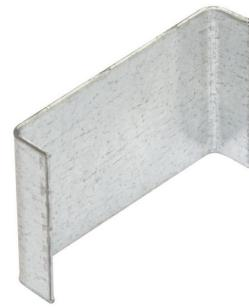
**Technical:****Product Type** Cable Retainer**Width** 50mm**Depth** 25mm**Weight** 0.01 Kgs**Material** Pre-Galvanised Steel (Zinc Coated)**Colour/Finish** Self Colour**Standards** BS EN 10346:2015**Important:**
