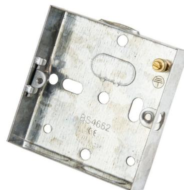
**Technical:****Product Type** Socket Box**Width** 75mm**Depth** 16mm**Height** 75mm**Weight** 0.07 Kgs**Number of Compartments****Number of Gangs** 1**Material** Pre-Galvanised Steel (Zinc Coated)**Colour/Finish** Self Colour**Standards** BS 4662:2006+A1:2009**Supplied With** 3 off 25mm x 12.5mm obround knockouts
