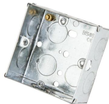
**Technical:****Product Type** Socket Box**Width** 75mm**Depth** 35mm**Height** 75mm**Weight** 0.12 Kgs**Number of Compartments****Number of Gangs** 1**Material** Pre-Galvanised Steel (Zinc Coated)**Colour/Finish** Self Colour**Standards** BS 4662:2006+A1:2009**Supplied With** 11 x 20mm knockouts
