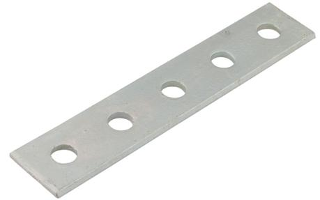
**Technical:****Product Type** Flat Plate**Weight** 0.36 Kgs**Gauge** 6mm**Material** Post Hot-Dipped Galvanised (HDG)**Colour/Finish** Self Colour**Standards** BS 6946:1988
