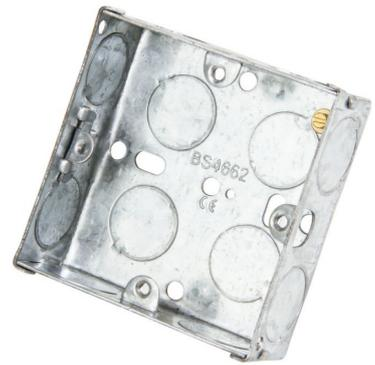
**Technical:****Product Type** Socket Box**Width** 75mm**Depth** 25mm**Height** 75mm**Weight** 0.10 Kgs**Number of Compartments****Number of Gangs** 1**Material** Pre-Galvanised Steel (Zinc Coated)**Colour/Finish** Self Colour**Standards** BS 4662:2006+A1:2009**Supplied With** 12 x 20mm knockouts
