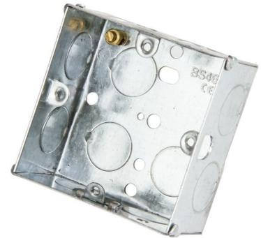
**Technical:****Product Type** Socket Box**Width** 75mm**Depth** 35mm**Height** 75mm**Weight** 0.12 Kgs**Number of Compartments****Number of Gangs** 1**Material** Pre-Galvanised Steel (Zinc Coated)**Colour/Finish** Self Colour**Standards** BS 4662:2006+A1:2009**Supplied With** 11 x 20mm knockouts
