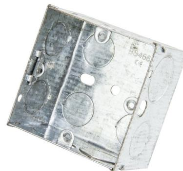
**Technical:****Product Type** Socket Box**Width** 75mm**Depth** 47mm**Height** 75mm**Weight** 0.15 Kgs**Number of Compartments****Number of Gangs** 1**Material** Pre-Galvanised Steel (Zinc Coated)**Colour/Finish** Self Colour**Standards** BS 4662:2006+A1:2009**Supplied With** 8 x 20mm knockouts 3 x 25mm knockouts
