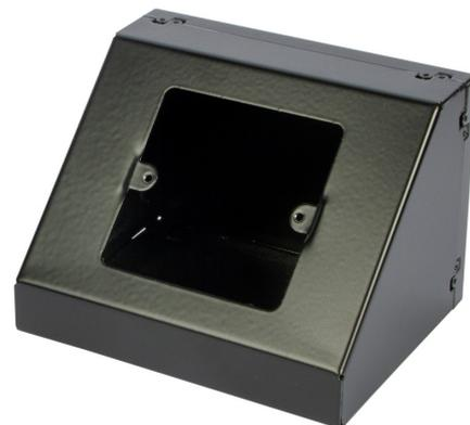
**Technical:****Product Type** Pedestal Boxes**Width** 130mm**Depth** 100mm**Height** 90mm**Weight** 0.41 Kgs**Dimensions** Overall Size: (D) 100mm x (W) 130mm X (H) 90mm**Angle** 45°**Number of Gangs** 1**Gauge** 1.0mm**Material** Pre-Galvanised Steel (Zinc Coated)**Colour/Finish** Black (RAL 9005)**Supplied With** 1 x 20mm knockout 1 x 25mm knockout Earth terminal in base
