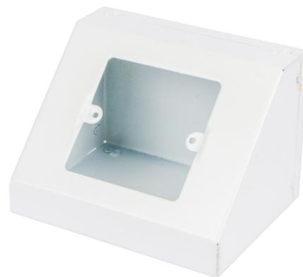
**Technical:****Product Type** Pedestal Boxes**Width** 130mm**Depth** 100mm**Height** 90mm**Weight** 0.41 Kgs**Dimensions** Overall Size: (D) 100mm x (W) 130mm X (H) 90mm**Angle** 45°**Number of Gangs** 1**Gauge** 1.0mm**Material** Pre-Galvanised Steel (Zinc Coated)**Colour/Finish** White (RAL 9016)**Supplied With** 1 x 20mm knockout 1 x 25mm knockout Earth terminal in base
