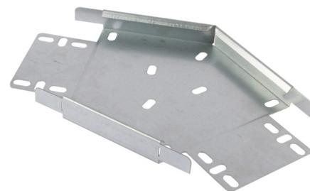
**Technical:****Product Type** Flat Bend**Width** 100mm**Height** 25mm**Weight** 0.35 Kgs**Angle** 45°**Gauge** Medium Duty**Material** Pre-Galvanised Steel (Zinc Coated)**Colour/Finish** Self Colour**Standards** BS EN 61537:2007; BS EN 10346:2015
