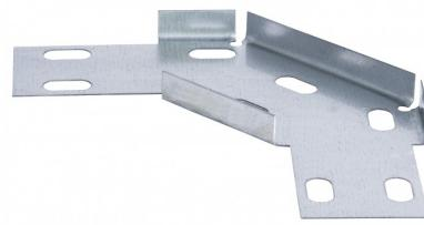
**Technical:****Product Type** Flat Bend**Width** 100mm**Height** 10mm**Weight** 0.20 Kgs**Angle** 90°**Gauge** Light Duty**Material** Pre-Galvanised Steel (Zinc Coated)**Colour/Finish** Self Colour**Standards** BS EN 61537:2007; BS EN 10346:2015**Pack Quantity** 1
