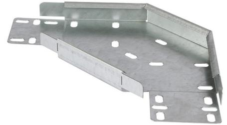
**Technical:****Product Type** Flat Bend**Width** 100mm**Height** 25mm**Weight** 0.35 Kgs**Angle** 90°**Gauge** Medium Duty**Material** Zinc Magnesium Steel ZM310**Colour/Finish** Self Colour**Standards** BS EN 61537:2007; BS EN 10346:2015
