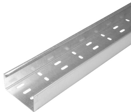
**Technical:****Product Type** Cable Tray**Width** 100mm**Height** 50mm**Length** 3000mm**Weight** 4.20 Kgs**Gauge** Heavy Duty**Material** Zinc Magnesium Steel ZM310**Colour/Finish** Self Colour**Standards** BS EN 61537:2007; BS EN 10346:2015
