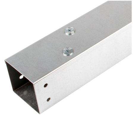
**Technical:****Product Type** Trunking**Width** 100mm**Height** 100mm**Length** 3000mm**Weight** 9.90 Kgs**Number of Compartments****Material** Pre-Galvanised Steel (Zinc Coated)**Colour/Finish** Self Colour**Standards** BS EN 50085-2-1 2006; BS EN 10346:2015**Supplied With** Turnbuckle lid fixings and coupler included.**Important:**
