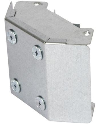
**Technical:****Product Type** Gusset Bend**Width** 100mm**Height** 50mm**Weight** 0.66 Kgs**Angle** 90°**Number of Compartments****Material** Pre-Galvanised Steel (Zinc Coated)**Colour/Finish** Self Colour**Standards** BS EN 50085-2-1 2006; BS EN 10346:2015**Trunking Weights:**
