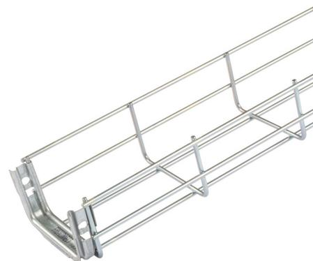
**Technical:****Product Type** Basket Tray**Width** 100mm**Height** 60mm**Length** 3000mm**Weight** 2.01 Kgs**Dimensions** 100 x 60mm mesh**Diameter** 3.9mm (Steel wire frame)**Outside Diameter** 3.9mm (Steel wire frame)**Material** Electro Zinc (E.Z)**Colour/Finish** Self Colour**Standards** BS EN 61537:2007**Supplied With** Pre-Installed FastConnect Coupler
