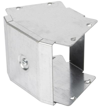
**Technical:****Product Type** Gusset Bend**Width** 100mm**Height** 100mm**Angle** 45°**Number of Compartments****Material** Pre-Galvanised Steel (Zinc Coated)**Colour/Finish** Self Colour**Standards** BS EN 50085-2-1 2006; BS EN 10346:2015
