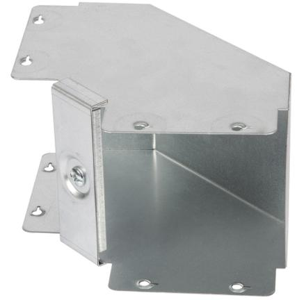
**Technical:****Product Type** Gusset Bend**Width** 100mm**Height** 100mm**Angle** 90°**Number of Compartments****Material** Pre-Galvanised Steel (Zinc Coated)**Colour/Finish** Self Colour**Standards** BS EN 50085-2-1 2006; BS EN 10346:2015
