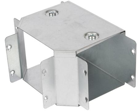
**Technical:****Product Type** Gusset Tee**Width** 100mm**Height** 100mm**Number of Compartments****Material** Pre-Galvanised Steel (Zinc Coated)**Colour/Finish** Self Colour**Standards** BS EN 50085-2-1 2006; BS EN 10346:2015
