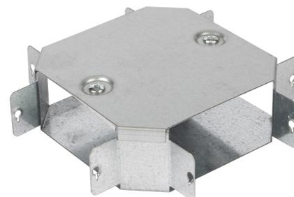
**Technical:****Product Type** Gusset Fourway**Width** 100mm**Height** 50mm**Number of Compartments****Material** Pre-Galvanised Steel (Zinc Coated)**Colour/Finish** Self Colour**Standards** BS EN 50085-2-1 2006; BS EN 10346:2015
