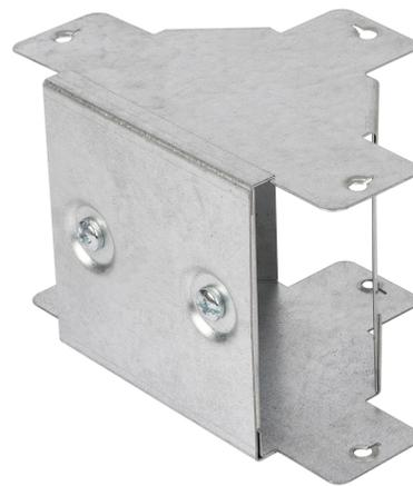
**Technical:****Product Type** Gusset Tee**Width** 100mm**Height** 50mm**Number of Compartments****Material** Pre-Galvanised Steel (Zinc Coated)**Colour/Finish** Self Colour**Standards** BS EN 50085-2-1 2006; BS EN 10346:2015
