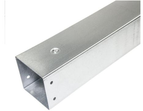
**BUY NOW****Technical:****Product Type** Trunking**Width** 100mm**Height** 100mm**Length** 3000mm**Weight** 9.00 Kgs**Number of Compartments****Material** Pre-Galvanised Steel (Zinc Coated)**Colour/Finish** Self Colour**Standards** BS EN 50085-2-1 2006; BS EN 10346:2015**Supplied With** Lid fixings and couplers included.**Important:**
