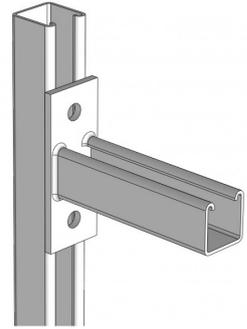
**Technical:****Product Type** Cantilever Arm**Width** 40mm**Height** 40mm**Length** 150mm**Weight** 0.74 Kgs**Gauge** 2.5mm**Material** Post Hot-Dipped Galvanised (HDG)**Colour/Finish** Self Colour**Standards** BS 6946:1988
