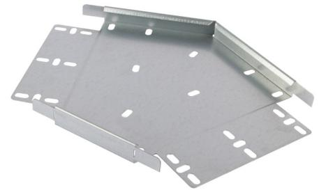
**Technical:****Product Type** Flat Bend**Width** 150mm**Height** 25mm**Weight** 0.52 Kgs**Angle** 45°**Gauge** Medium Duty**Material** Pre-Galvanised Steel (Zinc Coated)**Colour/Finish** Self Colour**Standards** BS EN 61537:2007; BS EN 10346:2015
