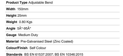
The approximate weights given are for pre-galvanised finish only, in kilograms (nominal) and subject to material thickness tolerance.
