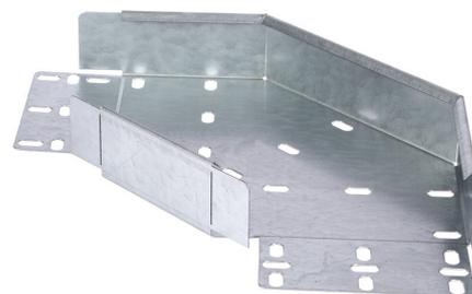
**Technical:****Product Type** Flat Bend**Width** 150mm**Height** 50mm**Weight** 0.64 Kgs**Angle** 90°**Gauge** Heavy Duty**Material** Pre-Galvanised Steel (Zinc Coated)**Colour/Finish** Self Colour**Standards** BS EN 61537:2007; BS EN 10346:2015
