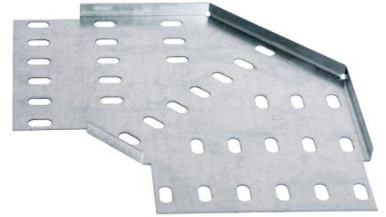
**Technical:****Product Type** Flat Bend**Width** 150mm**Height** 10mm**Weight** 0.34 Kgs**Angle** 90°**Gauge** Light Duty**Material** Pre-Galvanised Steel (Zinc Coated)**Colour/Finish** Self Colour**Standards** BS EN 61537:2007; BS EN 10346:2015**Pack Quantity** 1
