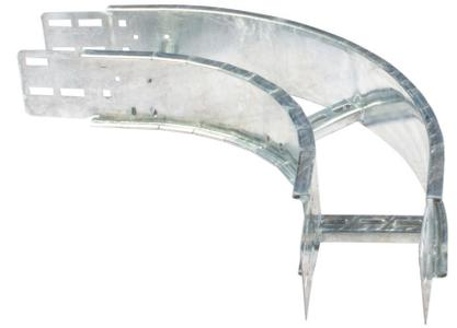
**Technical:****Product Type** Flat Bend**Width** 150mm**Height** 125mm**Weight** 4.30 Kgs**Angle** 90°**Diameter** 300mm Radius**Gauge** 1.5mm**Material** Post Hot-Dipped Galvanised (HDG)**Colour/Finish** Self Colour**Standards** BS EN ISO 1461:2009
