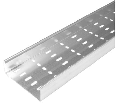
**Technical:****Product Type** Cable Tray**Width** 150mm**Height** 50mm**Length** 3000mm**Weight** 5.16 Kgs**Gauge** Heavy Duty**Material** Pre-Galvanised Steel (Zinc Coated)**Colour/Finish** Self Colour**Standards** BS EN 61537:2007; BS EN 10346:2015
