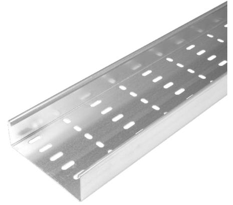
**Technical:****Product Type** Cable Tray**Width** 150mm**Height** 50mm**Length** 3000mm**Weight** 5.16 Kgs**Gauge** Heavy Duty**Material** Zinc Magnesium Steel ZM310**Colour/Finish** Self Colour**Standards** BS EN 61537:2007; BS EN 10346:2015
