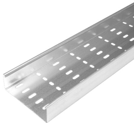
**Technical:****Product Type** Cable Tray**Width** 150mm**Height** 50mm**Length** 3000mm**Weight** 5.16 Kgs**Gauge** Heavy Duty**Material** Zinc Magnesium Steel ZM310**Colour/Finish** Self Colour**Standards** BS EN 61537:2007; BS EN 10346:2015
