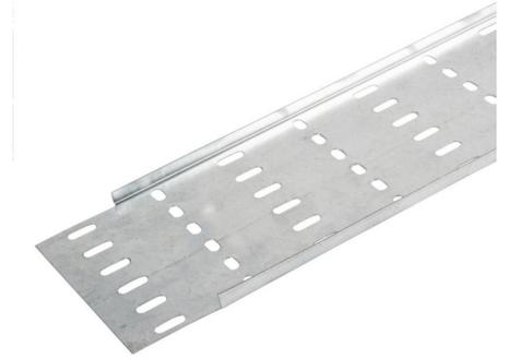
**Technical:****Product Type** Cable Tray**Width** 150mm**Height** 10mm**Length** 3000mm**Weight** 3.24 Kgs**Gauge** Light Duty**Material** Pre-Galvanised Steel (Zinc Coated)**Colour/Finish** Self Colour**Standards** BS EN 61537:2007; BS EN 10346:2015
