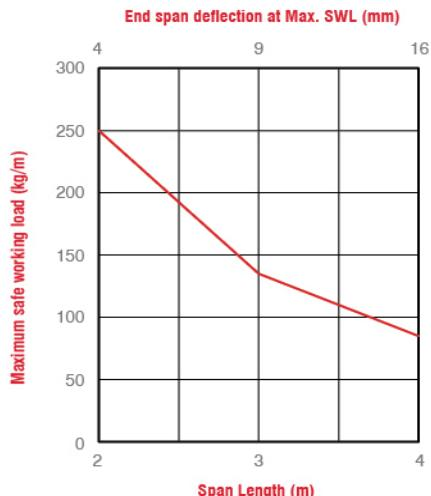
Graph showing safe working load vs span with deflections shown at SWL
