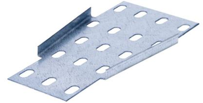
**Technical:****Product Type** Reducer**Width** 150mm**Height** 10mm**Weight** 0.55 Kgs**Gauge** Light Duty**Material** Zinc Magnesium Steel ZM310**Colour/Finish** Self Colour**Standards** BS EN 61537:2007; BS EN 10346:2015**Pack Quantity** 1
