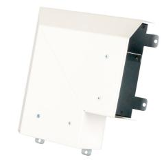
Product Type Flat Bend Depth 60mm Height 150mm Weight 1.52 Kgs Angle 90° **Number of Compartments** Gauge 1.2mm Lid +- Nominal Tolerance Material Pre-Galvanised Steel (Zinc Coated) Colour/Finish White (RAL 9016) **Standards** BS EN 10346:2015 Compliance Category 6a
