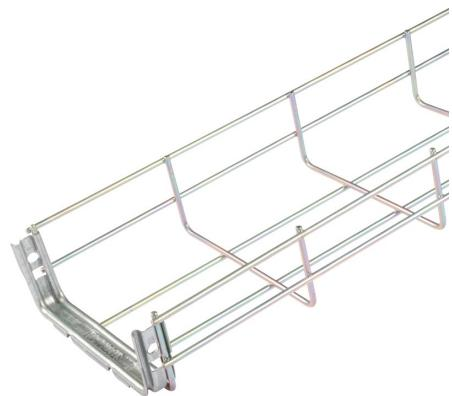
**Technical:****Product Type** Basket Tray**Width** 150mm**Height** 60mm**Length** 3000mm**Weight** 2.13 Kgs**Dimensions** 150 x 60mm mesh**Diameter** 3.9mm (Steel wire frame)**Outside Diameter** 3.9mm (Steel wire frame)**Material** Electro Zinc (E.Z)**Colour/Finish** Self Colour**Standards** BS EN 61537:2007**Supplied With** Pre-Installed FastConnect Coupler
