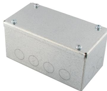
**Technical:****Product Type** Adaptable Box**Width** 150mm**Depth** 75mm**Height** 75mm**Weight** 0.52 Kgs**Material** Pre-Galvanised Steel (Zinc Coated)**Colour/Finish** Self Colour**Standards** BS EN 10346:2015**Supplied With** 20mm Knockouts
