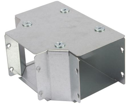
**IMAGE FOR ILLUSTRATIVE PURPOSES ONLY****Technical:****Product Type** Gusset Tee**Width** 150mm**Height** 50mm**Weight** 0.99 Kgs**Number of Compartments****Material** Pre-Galvanised Steel (Zinc Coated)**Colour/Finish** Self Colour**Standards** BS EN 50085-2-1 2006; BS EN 10346:2015**Trunking Weights:**
