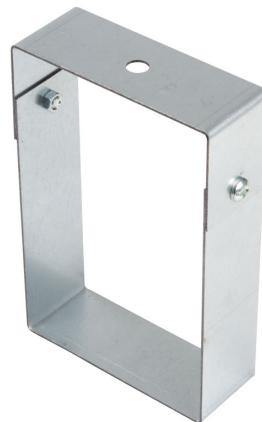
**Technical:****Product Type** Hanger**Width** 150mm**Depth** 45mm**Height** 150mm**Dimensions** Suspension Size (mm): W (50) x H (222)**Diameter** 11mm**Material** Pre-Galvanised Steel (Zinc Coated)**Colour/Finish** Self Colour**Standards** BS EN 50085-2-1 2006; BS EN 10346:2015**Supplied With** Bridge Pieces, Sleeve Couplers and M6 Screws**Pack Quantity** 4 Per Pack
