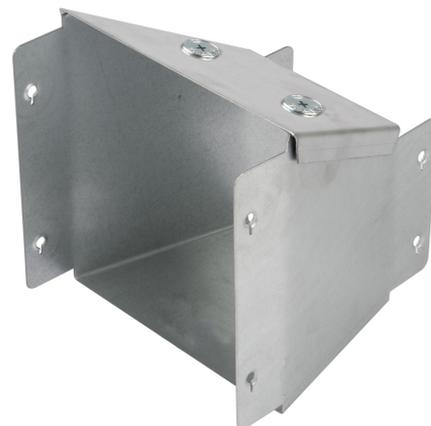
**Technical:****Product Type** Reducer**Width** Reduce 150mm x 150mm**Height** To 100mm x 100mm**Weight** 0.48 Kgs**Number of Compartments****Material** Pre-Galvanised Steel (Zinc Coated)**Colour/Finish** Self Colour**Standards** BS EN 50085-2-1 2006; BS EN 10346:2015**Trunking Weights:**
