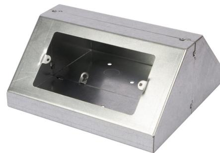
**Technical:****Product Type** Pedestal Boxes**Width** 190mm**Depth** 180mm**Height** 90mm**Weight** 0.70 Kgs**Dimensions** Overall Size: (D) 180mm x (W) 190mm X (H) 90mm**Angle** 45°**Number of Gangs** 2**Gauge** 1.0mm**Material** Pre-Galvanised Steel (Zinc Coated)**Colour/Finish** Self Colour**Supplied With** 1 x 20mm knockout 1 x 25mm knockout Earth terminal in base
