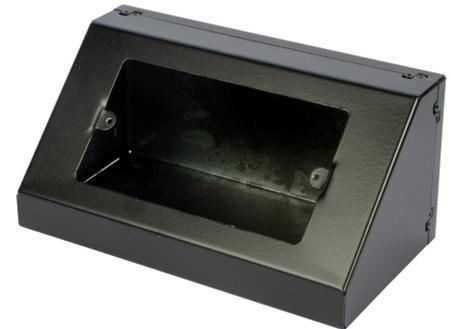
**Technical:****Product Type** Pedestal Boxes**Width** 190mm**Depth** 100mm**Height** 90mm**Weight** 0.54 Kgs**Dimensions** Overall Size: (D) 100mm x (W) 190mm X (H) 90mm**Angle** 45°**Number of Gangs** 2**Gauge** 1.0mm**Material** Pre-Galvanised Steel (Zinc Coated)**Colour/Finish** Black (RAL 9005)**Supplied With** 1 x 20mm knockout 1 x 25mm knockout Earth terminal in base
