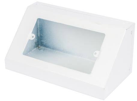
**Technical:****Product Type** Pedestal Boxes**Width** 190mm**Depth** 100mm**Height** 90mm**Weight** 0.54 Kgs**Dimensions** Overall Size: (D) 100mm x (W) 190mm X (H) 90mm**Angle** 45°**Number of Gangs** 2**Gauge** 1.0mm**Material** Pre-Galvanised Steel (Zinc Coated)**Colour/Finish** White (RAL 9016)**Supplied With** 1 x 20mm knockout 1 x 25mm knockout Earth terminal in base
