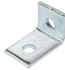
**Technical:****Product Type** Bracket**Weight** 0.13 Kgs**Dimensions** 40mm x 40mm**Angle** 90°**Gauge** 6mm**Material** Post Hot-Dipped Galvanised (HDG)**Colour/Finish** Self Colour**Standards** BS 6946:1988
