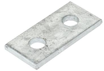
**Technical:****Product Type** Flat Plate**Weight** 0.14 Kgs**Gauge** 6mm**Material** Post Hot-Dipped Galvanised (HDG)**Colour/Finish** Self Colour**Standards** BS 6946:1988
