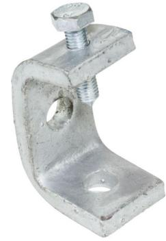
**Technical:****Product Type** Beam Clamp**Weight** 0.41 Kgs**Gauge** 6mm**Material** Post Hot-Dipped Galvanised (HDG)**Colour/Finish** Self Colour**Standards** BS 6946:1988**Supplied With** Cone pointed screw (TF050) supplied.
